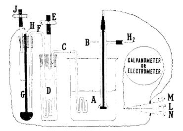
tube H, connection is made by means of a platinum wire with the lead or cadmium amalgam at the bottom of the electrode vessel G.
